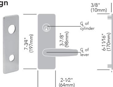
**Note:** The LS Escutcheon is not available with cylinder options: 10-63-, 11-60-, 11-63-, 11-64-, 60-, 63-, 64-, 70-, 72-, 73-, 65-73-, 65-73-7P-, 73-7P-, 81-, 82-, 83-, 84-, F1-82-, F1-82- & F1-83-. Also not available with electrified functions: 70, 71, 72, 73
