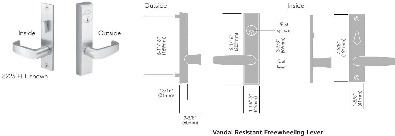
Note: Maximum projection varies by lever design. Largest projection is "A" lever – 3-9/16" (90mm)
