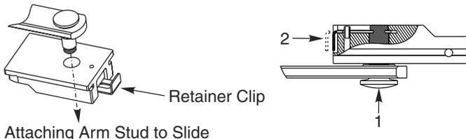
**Step 9:** Adjust closing power of unit (See Fig. 1) - Using a 1/8" allen wrench, turn the power adjustment shaft clockwise to increase door closing power. Door control is shipped set at midpoint of power setting. Maximum closing power can be achieved with 8 (360°) clockwise turns of the power adjustment screw.
