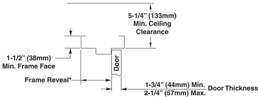
\*For frame reveals less than 3" (76mm) the arm adjusting rod can be field cut to a length of 9-1/2" (241mm) measured from centerline of connecting link bushing assembly.
