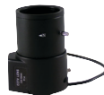
L-2.8-12DCIR (DAY & NIGHT) NEAR-INFRARED COMPATIBLE 1/3" FORMAT • DC AUTO-IRIS C/CS MOUNT • 6-60MM VARIOFOCAL F1.6 • SUPPORTS DAY-TO-NIGHT SURVEILLANCE ENSURES HIGH RESOLUTION PERFORMANCE
