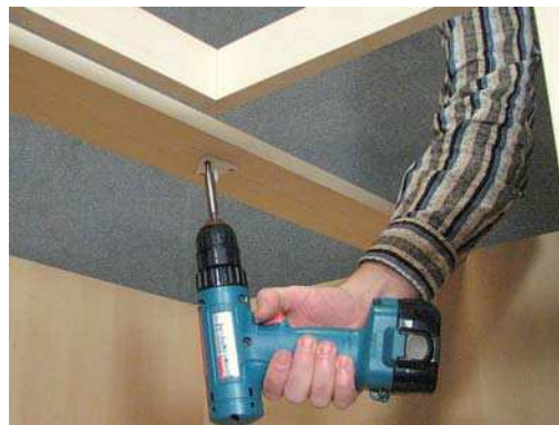
2. Screw the upper bearing
