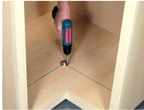
4. Mount the bottom bearing
