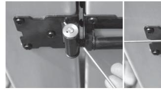
STEP 4 Rotate the bar back clockwise until the tension pin is against the hinge and remove bar.
