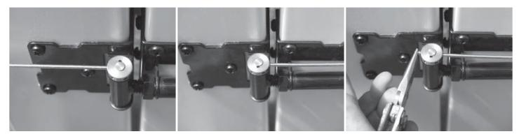
STEP 1 Insert the tension bar in hole at 9 o'clock position on tension wheel
