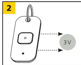
Replace 3 volt (CR2032) battery observing polarity and reassemble.
