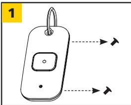
Remove back screws and disassemble.
