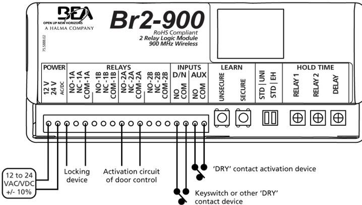
Relays 1 and 2 are DPDT: relays **1A and 1B** fire simultaneously and relays **2A and 2B** fire simultaneously.
