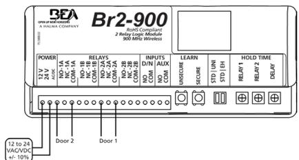
Door 2 will open and then Door 1 will open after a delay set by DELAY POT.
