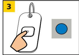
Press transmitter twice (white and blue LEDs on receiver will illuminate).
