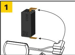
Connect transmitter<sup>1</sup> to push plate (NO and COM) and insert into box.
