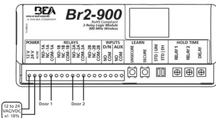
Door 1 will open and then Door 2 will open after a delay set by DELAY POT.
