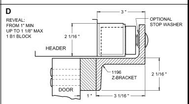
SPACER BLOCK IS THRU BOLTED TO DOOR USING THE BLOCK THRU BOLT PATTERN. Z-BRACKET IS THEN MOUNTED TO THE BLOCK, BY MEANS OF THE Z-BRACKET SCREWS AND THE TAPPED HOLES IN THE BLOCK.
