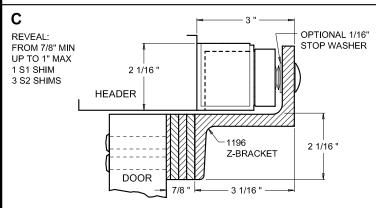
Z-BRACKET IS THRU-BOLTED TO DOOR USING THE Z-BRACKET TEMPLATE PATTERN. THE SCREWS PASS THROUGH THE SHIMS. SHIM STACKS OF 1/2" TO 7/8" USE LONGER 1 1/2" SCREWS FURNISHED WITH SHIMS.
