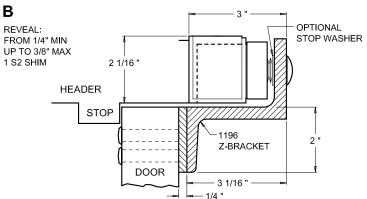
Z-BRACKET IS THRU-BOLTED TO DOOR USING THE Z-BRACKET TEMPLATE PATTERN. THE SCREWS PASS THROUGH THE SHIM.
