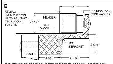
THE SECOND SPACER BLOCK IS THRU BOLTED TO DOOR USING THE BLOCK THRU BOLT PATTERN, WITH THE SCREWS PASSING THROUGH THE FIRST BLOCK. Z-BRACKET IS THEN MOUNTED TO THE SECOND BLOCK, USING THE TAPPED HOLES, WITH THE APPROPRIATE LENGTH SCREWS PASSING THOUGH THE SHIM.
