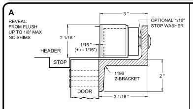
Z-BRACKET IS THRU-BOLTED TO DOOR USING THE Z-BRACKET TEMPLATE PATTERN.
