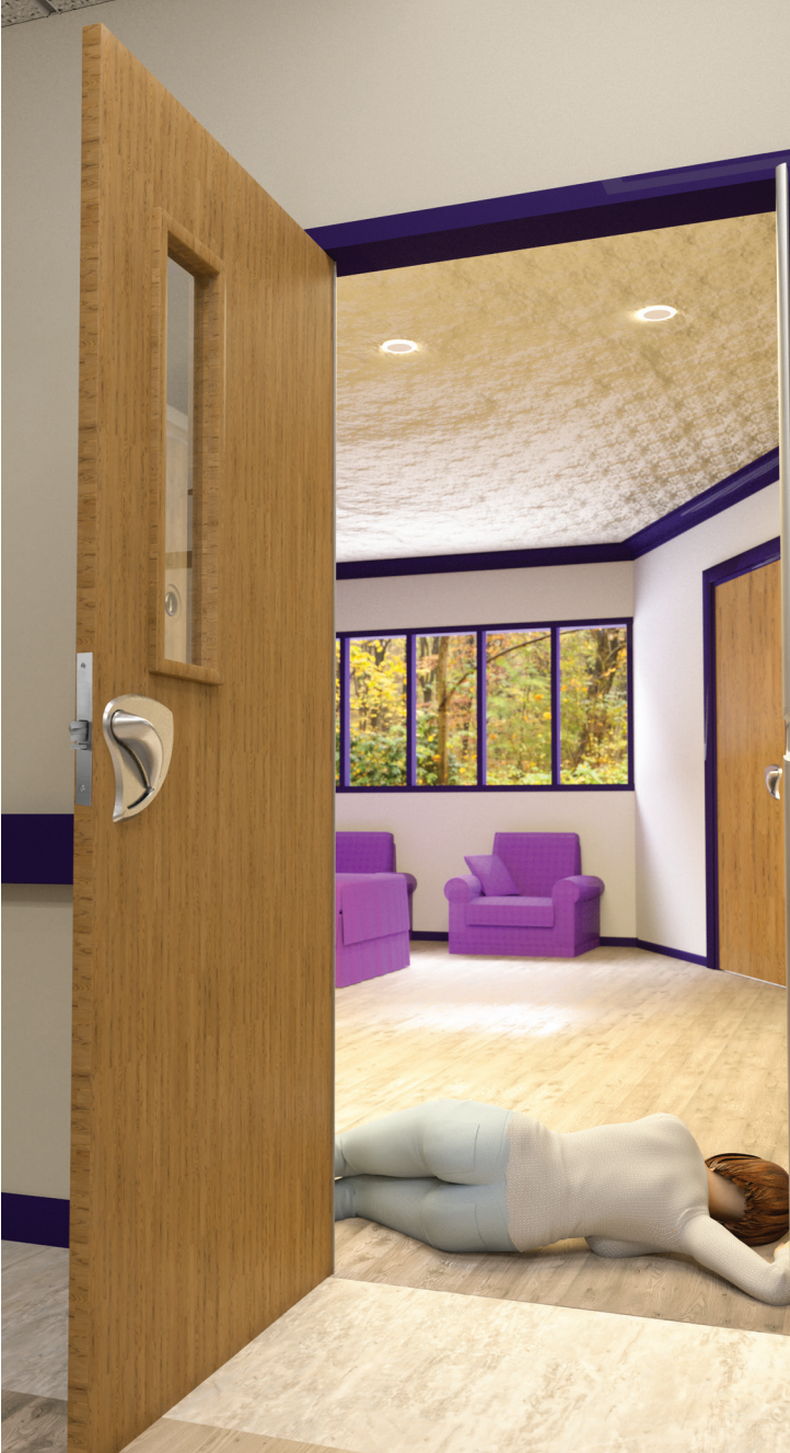
4. Door opens outward in the opposite direction to allow quick and easy access to the patient
