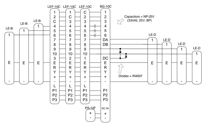
For best results, Aiphone recomends the use of wire #822220 between LEF-10C's, LEF -1C's and to the all call adaptor. Wire #822203 to the door. Maximum overall distance of 69 0 feet.
