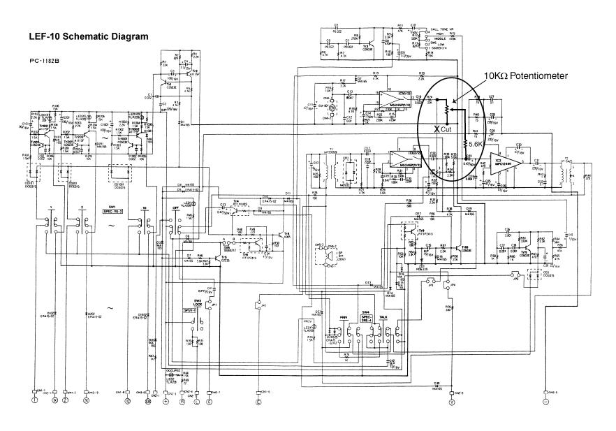
Add components as shown above. Cut trace where marked with an X. Potentiometer will lower outgoing volume. Main volume control on the master station will control the overall volume in both directions.
