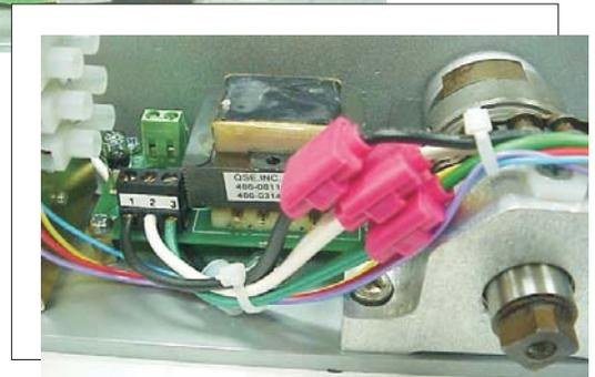
**Step 6.** Mount 433MHz Receiver to unit as shown using Velcro strip provided
