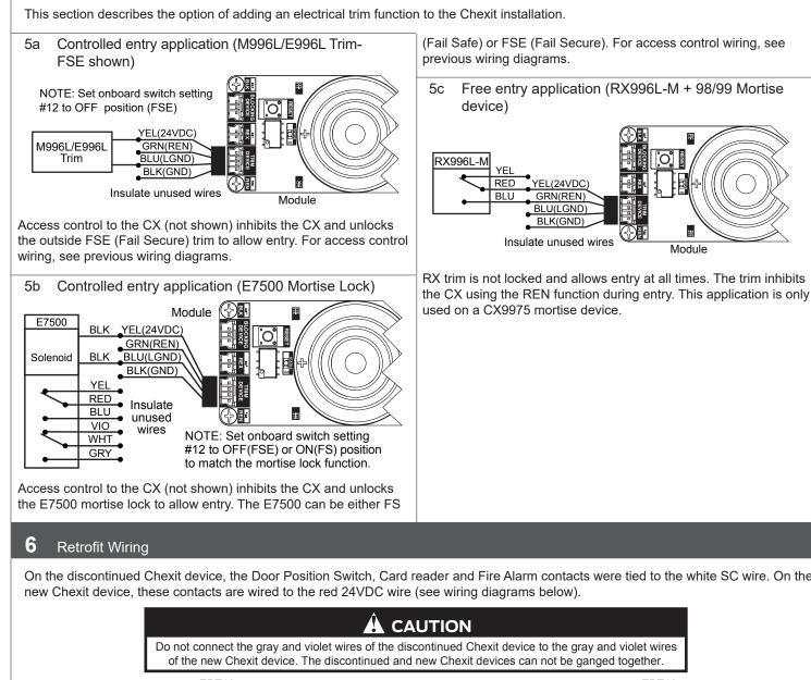
On the discontinued Chexit device, the Door Position Switch, Card reader and Fire Alarm contacts were tied to the white SC wire. On the
