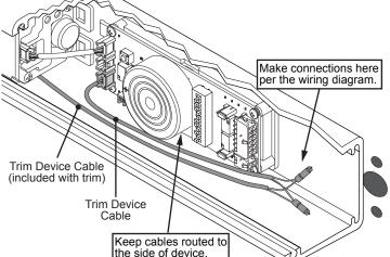
If using electric mortise lock (E7500 or SS7500 monitor mortise lock), install lock per instructions included with lock. Route lock wires through the door as shown.
