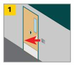
Remove existing touch pushplate and disconnect two (2) existing in-wall wires from pushplate and door control activation.
