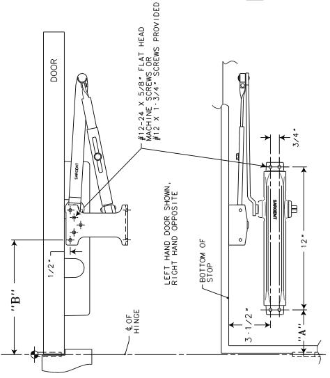
TEMPLATE A7750. REINFORCE METAL DOORS AND FRAMES PER ANSI A250.8 AND SDI-100 STANDARDS, 12 GAUGE RECOMMENDED. SEE THIN TOP RAIL DOORS, USE 1331-D PLATE. NOTES FOR
