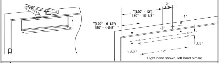
With provided fasteners, install foot to frame and secure closer body to door with power adjustment away from hinge
