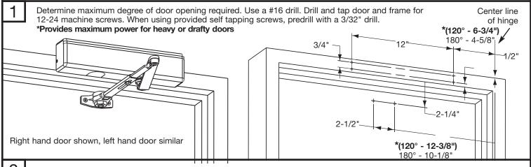
With provided fasteners, install foot to door as shown and closer body to frame with power adjustment away from hinge
