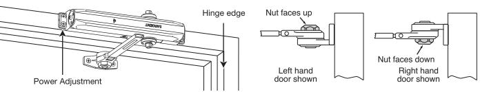
On both right and left hand doors, secure main arm to spindle with screw and washer provided. Align flat mark as shown
