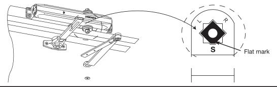
Open door and insert foot into main arm. Close door fully, and while pushing arm as shown in picture, tighten arm bolt
