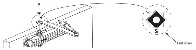
Open door and insert foot into main arm. Close door fully, and while pushing arm as shown in picture, tighten arm bolt
