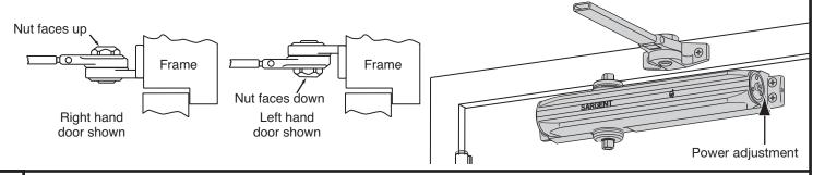
3 On both right and left hand doors, secure main arm to top spindle with screw and washer provided. Align flat mark as shown
