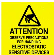
Circuit board components are vulnerable to damage by electrostatic discharge (ESD). ESD can cause immediate or subtle damage to sensitive electronic parts. An electrostatic charge can build up on the human body and then discharge when you touch a board. A discharge can be produced when walking across a carpet and touching a board, for example. Before handling any board, make sure you dissipate your body's charge.
