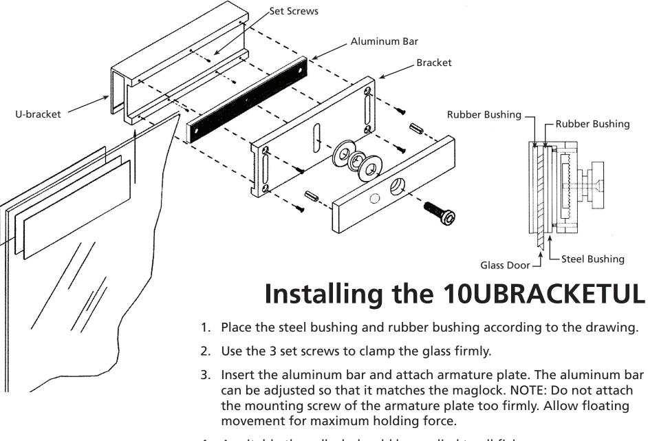
4. A suitable threadlock should be applied to all fixing screws.
