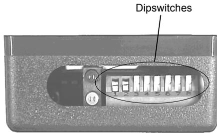
Set the dipswitches according to the chart below to achieve the desired lock out time delay. The dipswitches are configured to send a binary coded input to the microprocessor to establish the correct lock out time delay.
