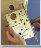
Without opening lock case, rotate latchbolt 180 degrees and allow it to retract back into case.
