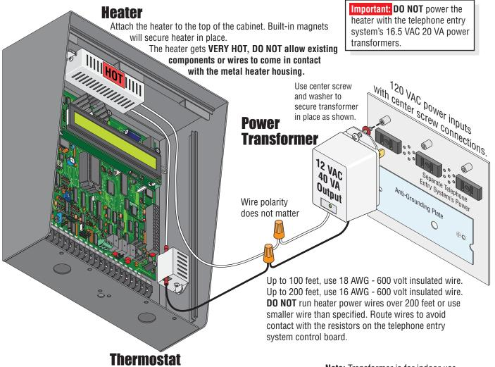
Attach the thermostat on the side near the bottom of the cabinet **as far from heater as possible. DO NOT position the thermostat right next to the heater.** Built-in magnets will secure thermostat in place. Thermostat will automatically turn heater on at approximately 40°F (4°C) and off at 55°F (12°C). **Note:** Transformer is for indoor use and **MUST** be in a protected enclosure from weather when using outdoors.
