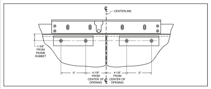
2. From the illustrations below select the one that resembles your door type and follow the instructions for drilling the armature mounting bracket screw holes.
