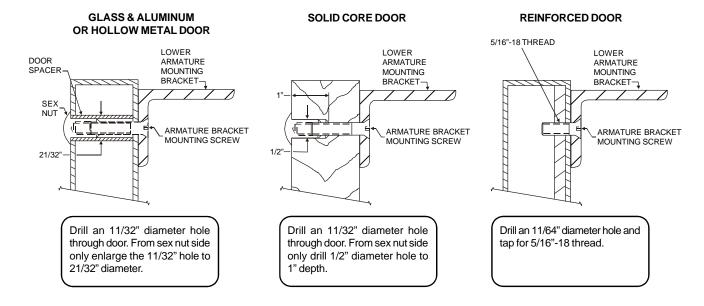
3. Mount the armature and mounting bracket assembly to each door using the appropriate hardware for you door type. Frimly tighten the mounting screws with a 3/16" hex wrench.
