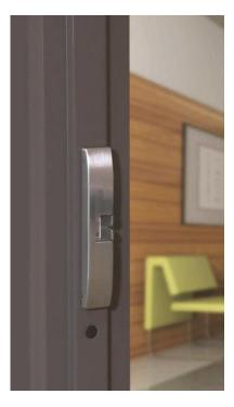
The HES 9600 series is a windstorm rated, surface mounted electric strike designed to accommodate rim exit devices with a 3/4" throw latchbolt. All components are completely encased within its 3/4" thick stainless steel housing, no cutting on the frame is required for installation.
