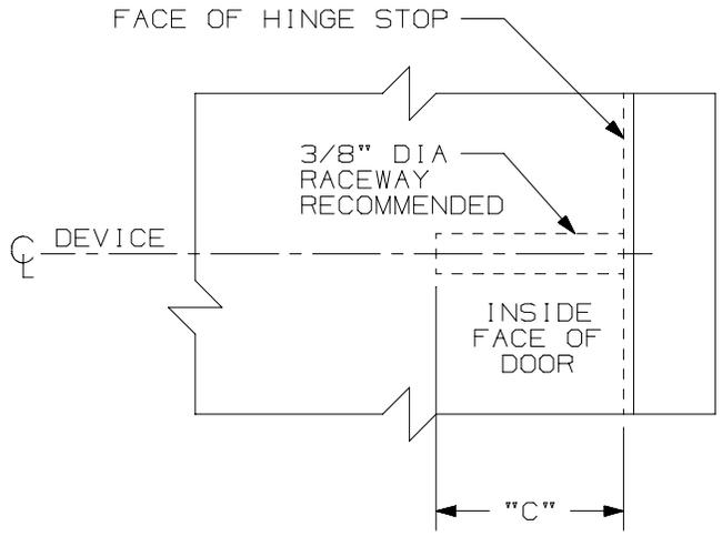
NOTE: MOUNTING HOLES TO BE PREPARED AT INSTALLATION ON DOOR.
