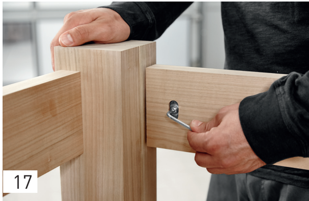
17 Tighten the connection using a 4 mm hex wrench.
