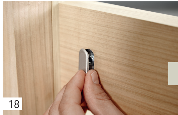
18 Optionally, you can cover the mortise with a cover cap, available in one of three colors depending on the material: silver, light brown or dark brown.
