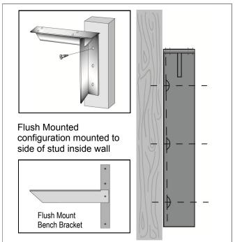
**Installation Note:** To minimize shimming, be sure to install the brackets so that the supporting arm is parallel to the floor. Install so that the vertical support is flush with, or slightly behind the stud to allow for application of sheet rock. Left hand and Vertical Flush Mount brackets are available.
