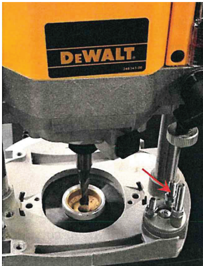
Short stop/deepest cut (42 mm) with stop bar pushed in as shown in Fig. 12.
