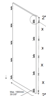
Preparation of wall panels with clips
