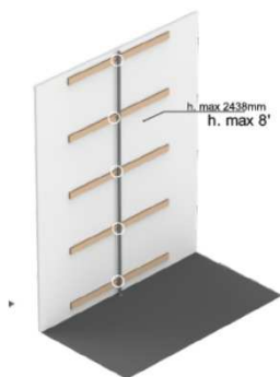
Adding wooden nailing strips
