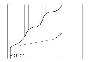
**Step 2:** Along the line locate the location of the wood studs behind the wall and mark the center line of the studs on the line. Hold the *Wood Mounting Plate* on the wall in the desired location and transfer the stud center lines to the *Wood Mounting Plate*.
