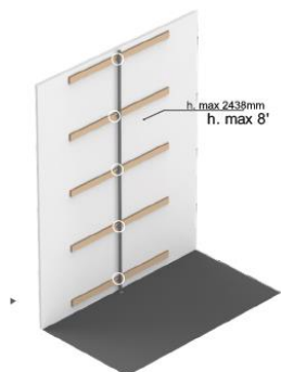
Adding wooden nailing strips
