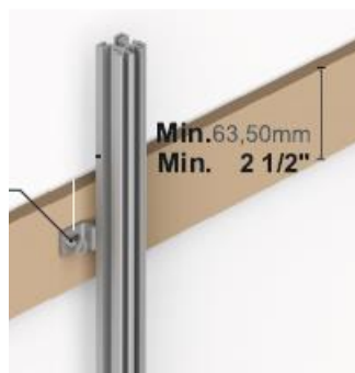
Installation of profiles on wall
