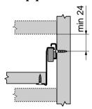
In addition, the new MINIFIX was modified so that the reference point is not the drawer base bottom anymore but the minimum installation distance.
