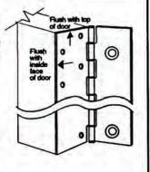
NOTE: Fasten top most screw first, and bottom most screw second making sure that hinge is aligned correctly.
