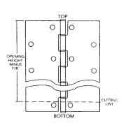
DOUBLE CHECK MEASUREMENT BEFORE CUTTING! NOTE: cut end of hinge must be used as **BOTTOM OF HINGE ONLY!**
