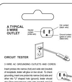
glow.Then test between wide side (neutral) and "U" shaped hole.tester should not glow.
