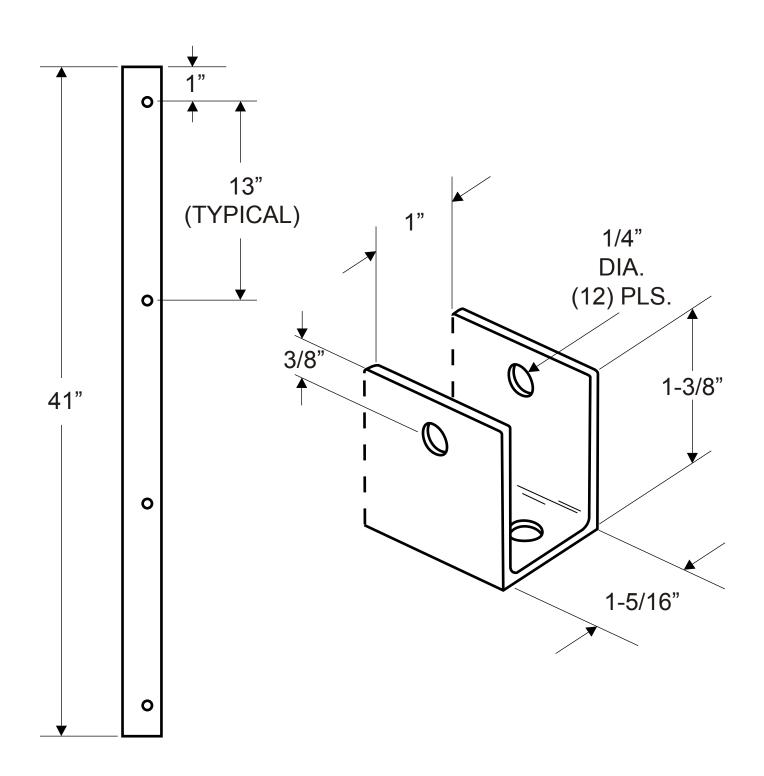
NOTE: ALL WALL THICKNESS AT 1/8" FOUR HOLES IN BASE
