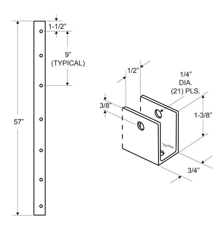
NOTE: ALL WALL THICKNESS AT 1/8" SEVEN HOLES IN BASE
