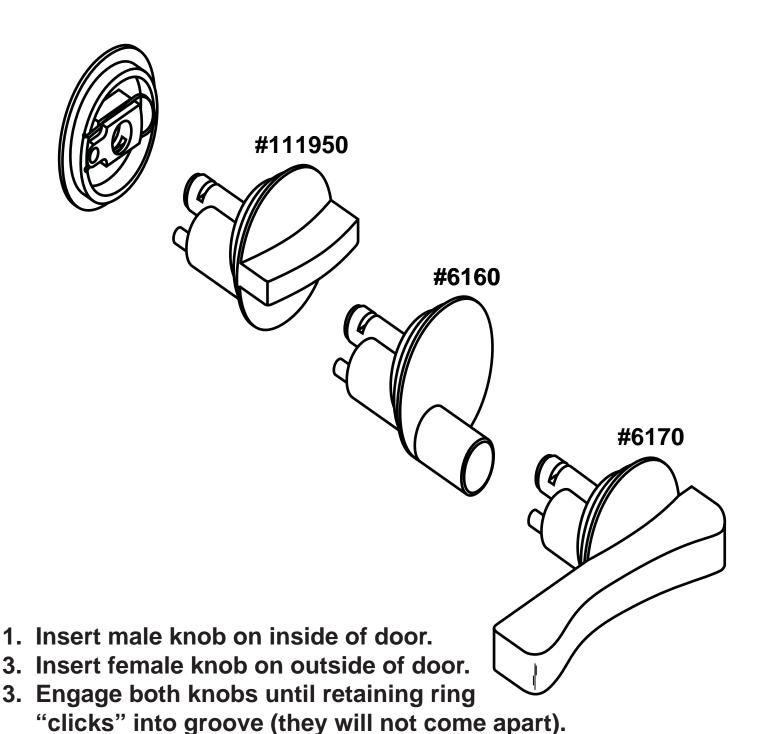
REMOVAL - To remove latch, drill 3/8" diameter hole through center of female knob (outside) 5/8" deep. Pull knob set apart.
