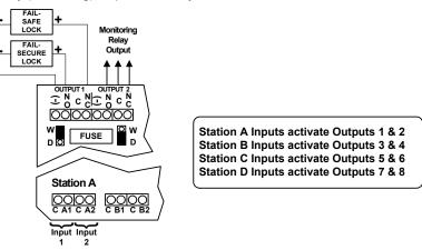
Activating each station's Input 1 OR Input 2 will trigger the corresponding lock output AND the monitoring output simultaneously.
