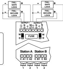
Each input may be individually configured to operate as a conventional relay or a time delayed relay. Alternatively, each input may be individually configured to operate as a latching relay or a time delayed relay.
