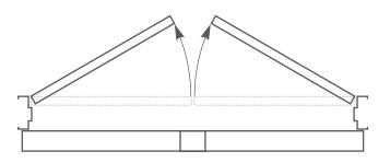
D6021/D6031/D6061/D6071 Series Operator mounted on Push Side Left Hand/Right Hand Outswing Doors
