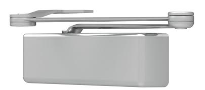
The 4110 is LCN's best performing heavy duty closer with an adjustable spring and possible hold open point beyond 140 degrees, meeting ADA requirements. Backed by a 30 year warranty, the cast iron body and all weather fluid offer versatility in high traffic applications.
