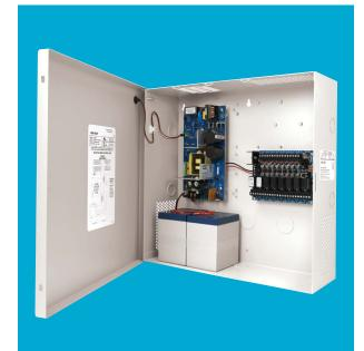
The Securitron AQS2410 Series of switching power supplies are single voltage, UL listed, supervised units with a dedicated battery charging circuit. They provide 10 Amps at 24VDC, with up to 16 independently controlled power limited outputs.
