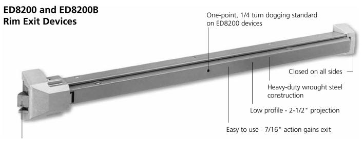
3/4" throw stainless steel pullman-type latchbolt with stainless steel auxiliary deadlocking latch standard
