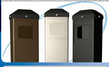
The Bollard is used for mounting pushplates that activate automatic doors. It will accept BEA's 4 1/2" Square Pushplate, 4 3/4" Square Pushplate, 4 3/4" Panther Pushplate, Dual Vestibule Pushplate and 4 1/2" Round Pushplate. The post is made of durable carbon steel and the mounting bracket is made of stainless steel for strength. It can be mounted on either existing concrete or newly poured concrete.
