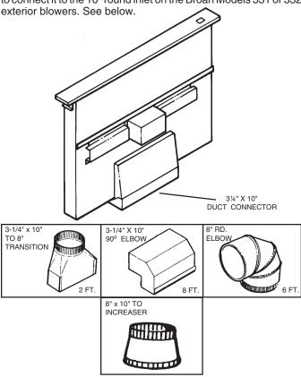
The system will operate most efficiently when the ductwork does not exceed 40 feet of equivalent duct. The illustrations above, show equivalent feet of elbows and transitions. The number of feet of straight 3-1/4" x 10" or 6" duct plus the equivalent feet of elbows or transitions to be used should equal 40 feet or less.
