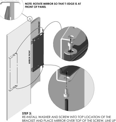
HOLES ON BOTTOM AND INSTALL SCREW THROUGH
