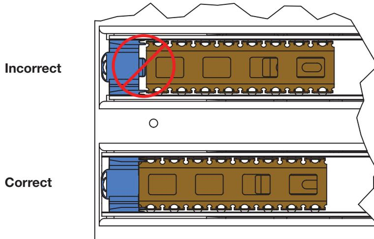
**Warning:** Ensure racks are properly attached to their slides and operating smoothly prior to filling racks to avoid injury from tipping during use.
