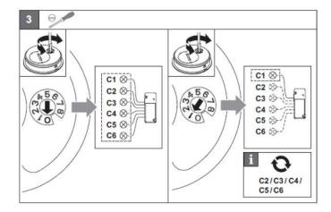
Test the pairing by pressing the power button for on and off. [Turning the dial to 0 for all zones or individual zones (C1, C2, C3... 1, 2, 3...) (Dial position 1 = C1 etc., Dial position 0 = all zones)]. Note: C1 will turn all C1 lights on /off etc.
