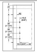
Mounting position of the Free swing fitting on the door; indications are for Full Overlay Door Bracket
