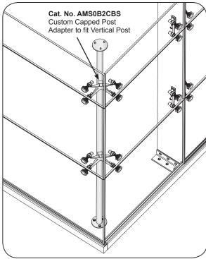
The Glass panels above are mounted to a CRL 4-Way Arm 90 Degree Heavy Duty Post Mount Fitting called PMH490BS which is meant to hold 90 degree glass panels at the corner of the glass wall. The Spider comes with M16-2.0 x 99.5 mm stainless steel threaded stud. A custom Post Adapter Cat. No. AMS0B2CBS can be used to fit the Round Vertical Post.
