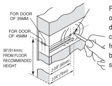
Place template on outside of door with height center line 36" from floor. Mark both holes as shown.
