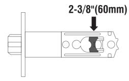
The latch is set 2-3/8"(60mm) To adjust to 2-3/4"(70mm), Slide Spindle cam to 2-3/4" markings.
