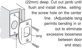
flush and install strike, setting the screw hole on the center line. (Adjustable tang permits bending in or out to eliminate excessive looseness between door and stop).
