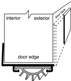
3. Slide door bottom shoe in place and close door. Position so that it makes light even contact with the threshold. Mark door in center of slotted holes.
