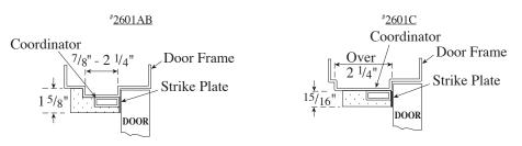
NOTE: Field adjustment of door closers is required after installation of coordinator to insure against doors closing too fast and changing coordinator mechanism. Field adjustment of coordinator override could be needed.
