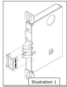
Slide bracket over latch as shown. Bracket will be secured when faceplate is installed.
