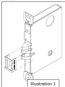
Slide bracket over latch as shown. Bracket will be secured when faceplate is installed.
